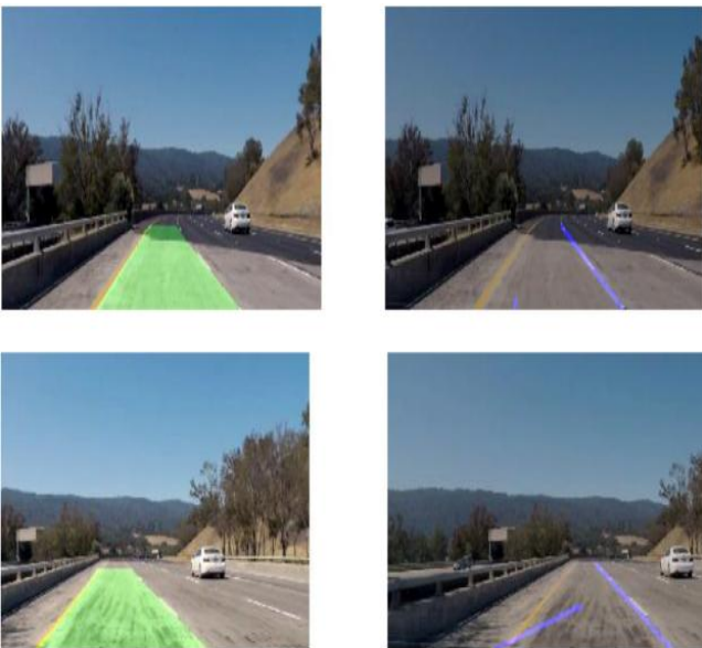
Fig.4a.Result of the proposed lane-finding algorithm compared with that of the conventional algorithm. The accompanying example exhibits the suggested algorithm's resistance to changes in illumination and road surface. When compared to the previous basic method, the suggested sanity tests and filtering algorithms appear to be more resilient. The revised perspective-transform-based
