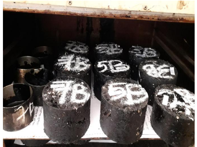
Fig. 4 the specimens at oven for five days at 85°C
