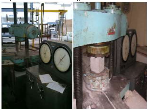
UTM where cubes are tested for compressive strength
