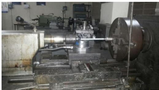
Figure 3: Tool Dynamometer set-up
