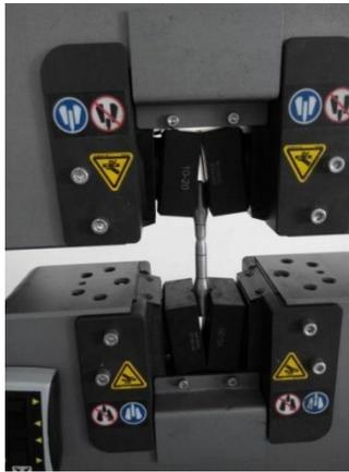
Figure 2: 400 kN Instron make UTM
