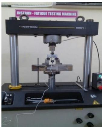
Figure 4: Fracture toughness experiment on 100 kN Instron
