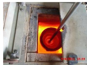
Figure 1: Stir casting machine
