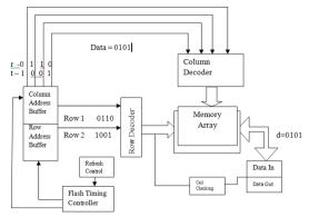
There are two locators i.e., column address and row address buffer which are send the files to the column decoder and row decoder respectively. Further, they will be sent to the memory array which is indicated as columns and rows as 0110 & 1001 respectively.
