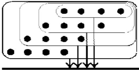
Fig.5.Row by row addition in a sequential multiplier.
