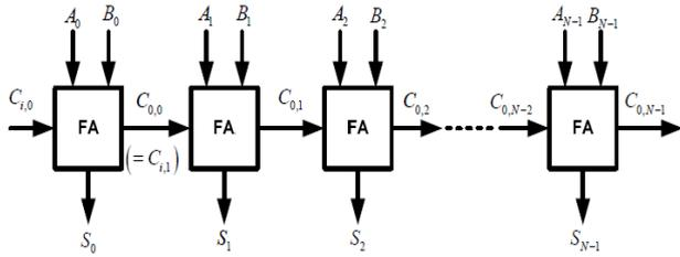
Fig.7. The N-bit Ripple Carry Adder constructed by N set single bit Full-adder
