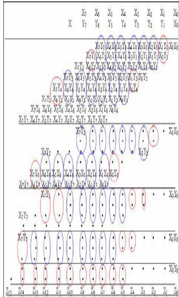
Fig.4.6 bit×6 bit Wallace tree multiplier.
