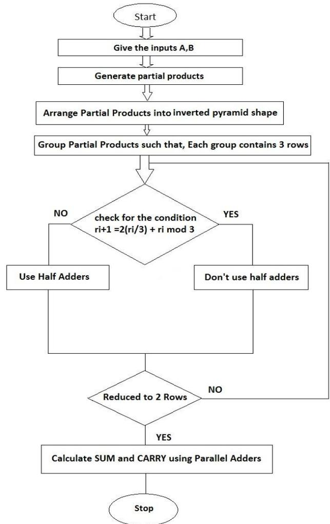
Fig.2.Flow chart for Modified Wallace Multiplier A.Mac Operation.
