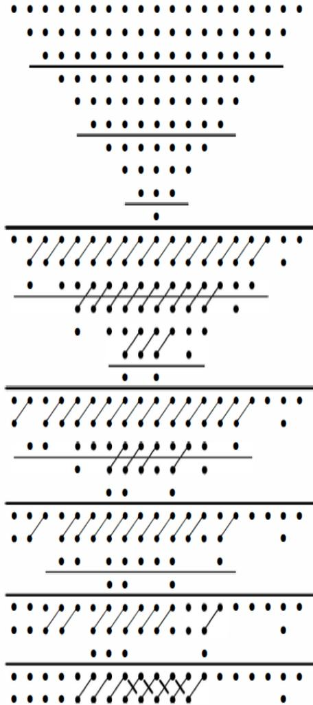
Fig.1.Modified Wallace 10-bit by 10-bit reduction.
