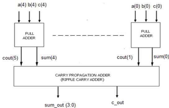
Fig.6.4-bit Carry Save Adder.
