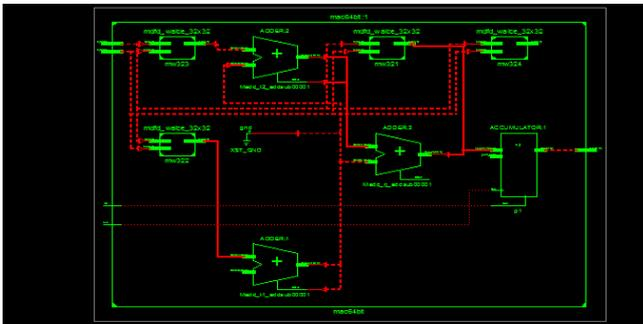
Fig.9. RTL Schematics of internal modules of MAC64 bit
